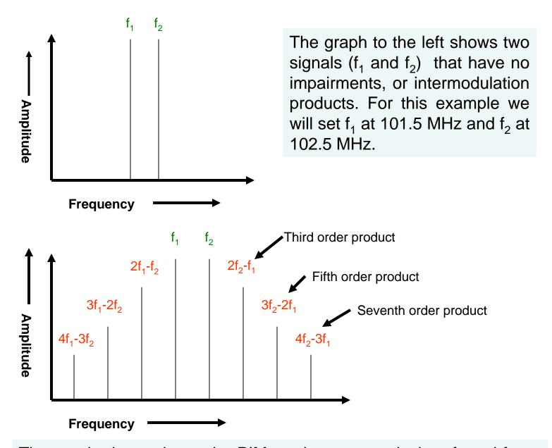
The graph above shows the PIM products created when  $f_1$  and  $f_2$  are subjected to a non-linearity. The first PIM product on either side of the two desired signals is called a third order mixing product, the second signal is a fifth order mixing product. Note: The mixing products shown on the graph are not drawn to any particular scale.
