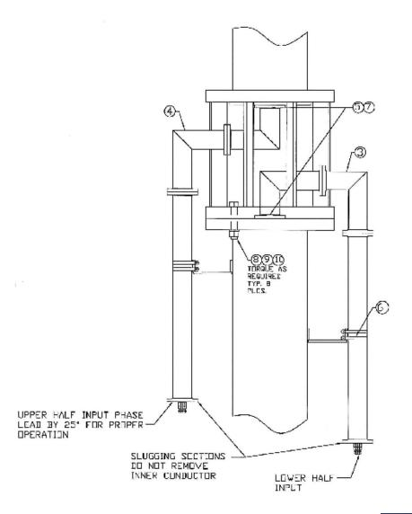
This is a drawing of the dual feed system wedding cake. There three were goals that had to be met first here. The and most mechanical important is strength. The second having enough room inside the wedding cake to install the EIA flanged components inside. The third was the length of the wedding cake to proper spacing ensure between the slots of both halves of the antennas, as this affects the elevation pattern when run as a single antenna array.
